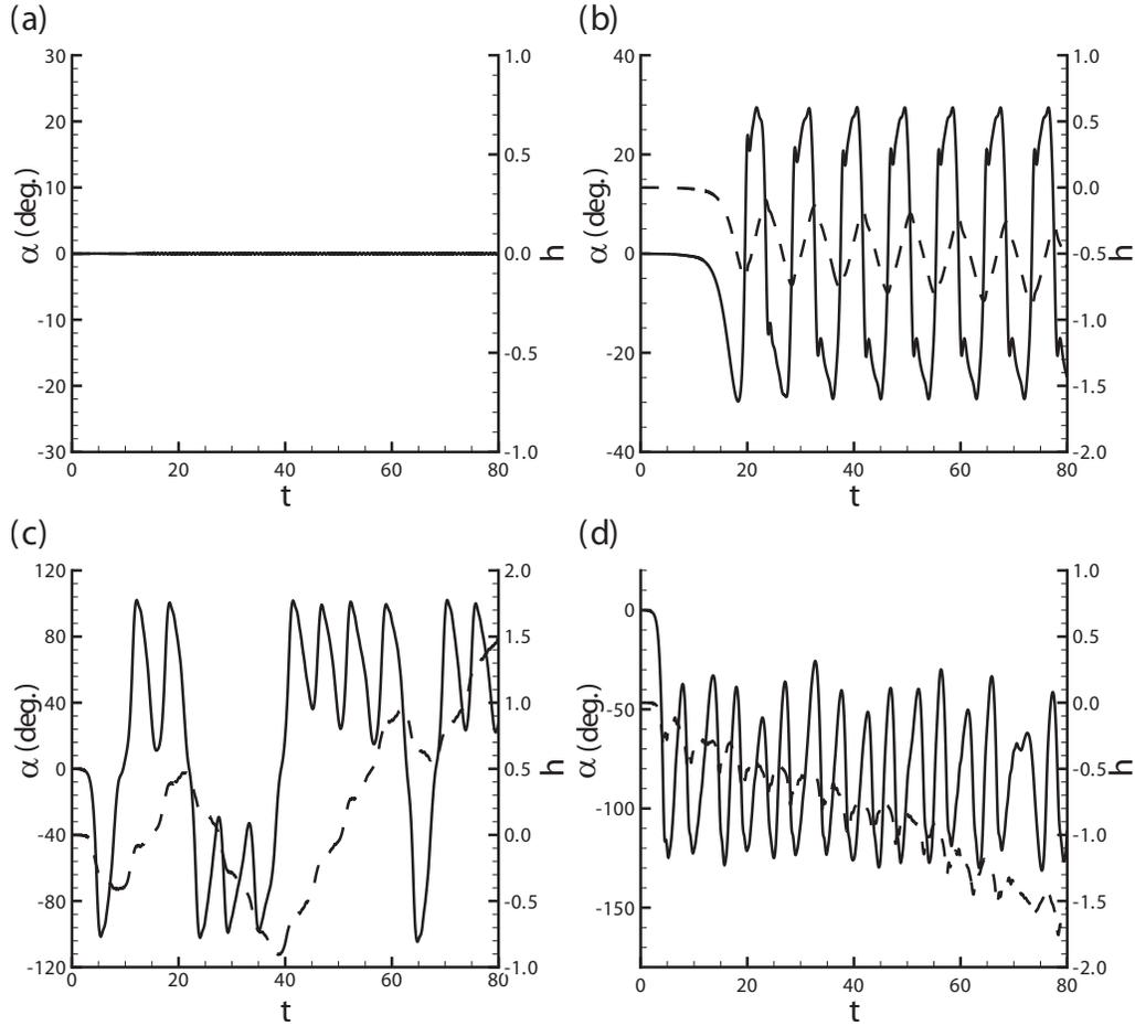
FIG. 3. Variations of the angle of attack  $\alpha$  (solid lines) and heave  $h$  (dashed lines) at four different cases: (a)  $b=-0.2$ ,  $k_\alpha=0.1$ ; (b)  $b=-0.2$ ,  $k_\alpha=0$ ; (c)  $b=0$ ,  $k_\alpha=0.012$ ; and (d)  $b=0$ ,  $k_\alpha=0$ .
