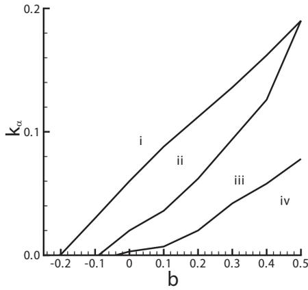
FIG. 6. Boundaries between the four system behaviors: (i) steady state at  $\alpha=0$ , (ii) periodic oscillations around  $\alpha=0$ , (iii) mode switching between oscillations around  $\alpha_0$  and  $-\alpha_0$ , and (iv) oscillations around  $\alpha_0$  ( $\alpha_0 \neq 0$ ).
