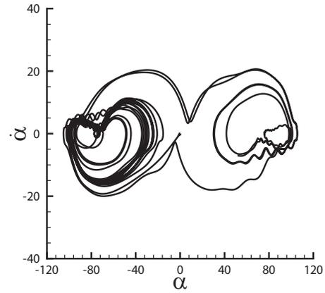
FIG. 8. Projection of the phase plane trajectory in the  $\alpha$ - $\dot{\alpha}$  plane showing competition between two oscillation modes.  $b=-0.05$  and  $k_\alpha=0$ . The angles are shown in degrees.
