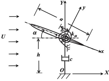
FIG. 1. Schematic of the flapping foil energy harvester.
